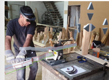
AR model guides the craftsman in bending
